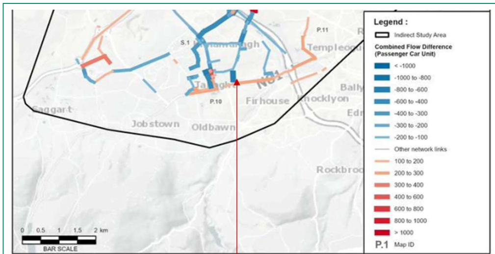
Diagram 6.41: Flow Difference on Road Links (Do Minimum vs. Do Something), PM Peak, 2028 Opening Year
