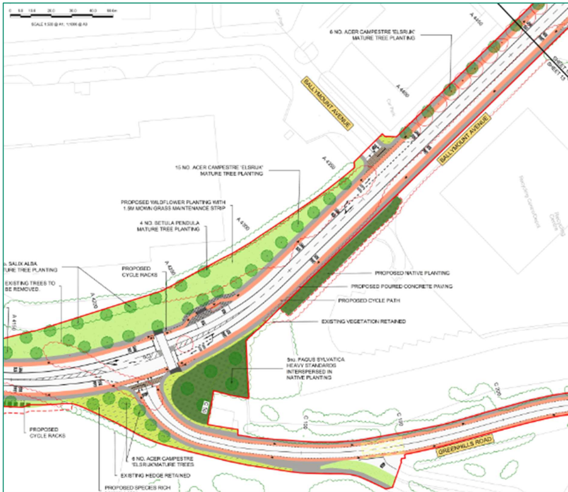
Figure 2.8.11.42: Extract of Landscaping General Arrangement Drawings along Ballymount Avenue from its junction with Greenhills Road
