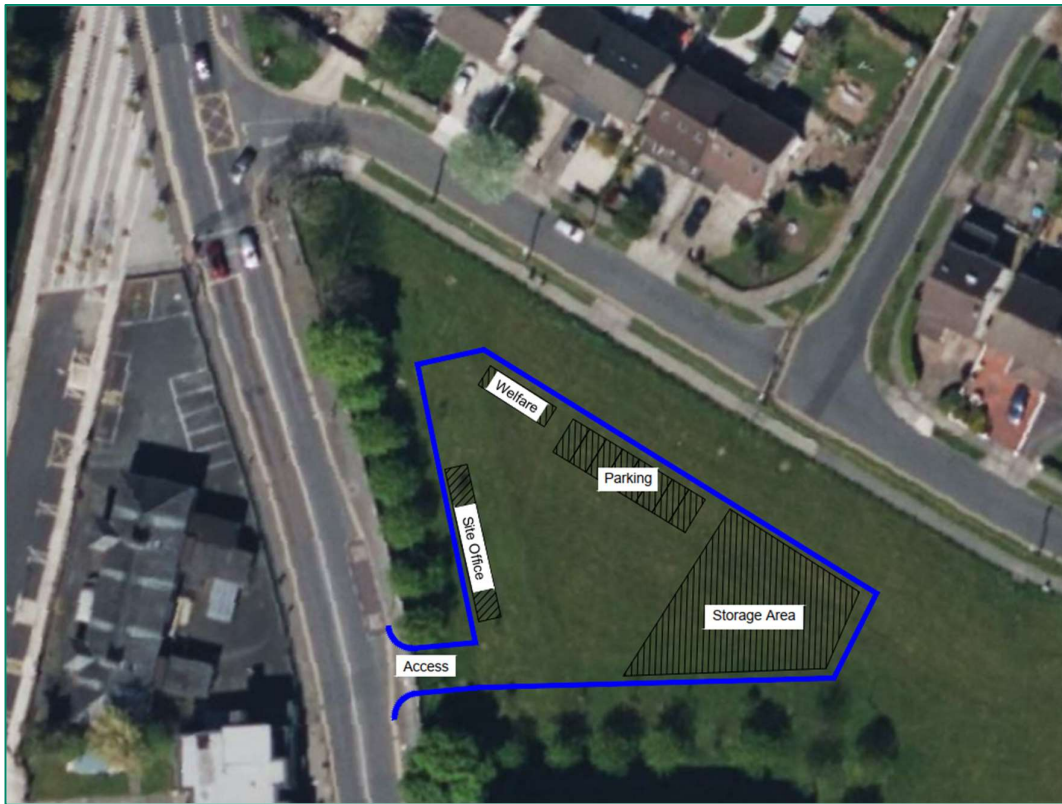
Figure 2.1.3: Site Compound TC2 Aerial Image Overlay (Image Source: Goggle)
