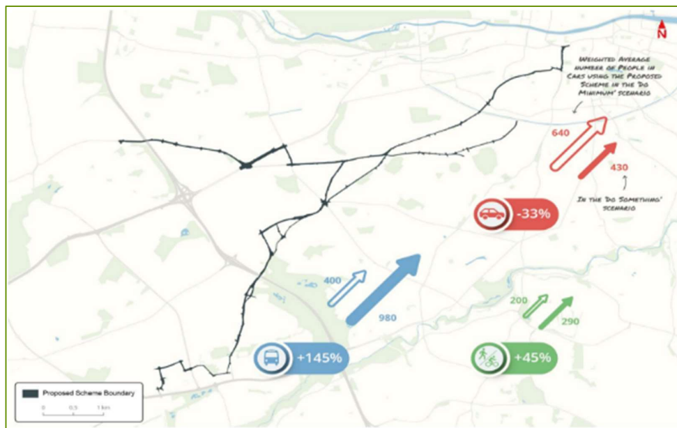
Figure 2.4.8: People Movement by Mode travelling along the Proposed Scheme during 2028 AM Peak Hour (Diagram 6.6 in EIAR Chapter 6)
