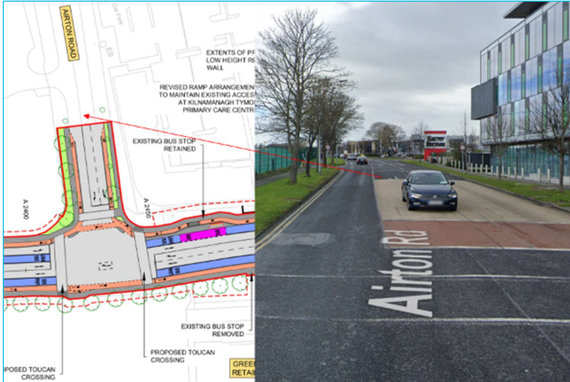
Figure 2.8.11.6: Extract of General Arrangement Drawings at Airton Road and Existing View of Airton Road (Image source: Google)
