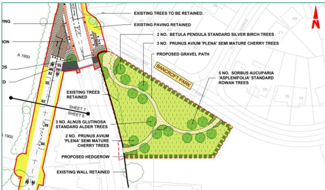
Figure 2.8.11.3 Extract from Landscaping General Arrangement Drawings from Figures: Part 1 of 3 of Volume 3 of the EIAR
