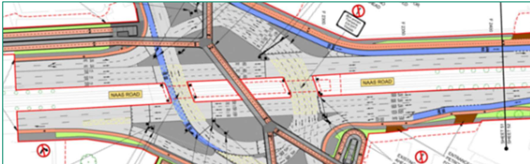
Figure 2.8.8.11 Interface with Red Luas Line at Naas Road / New Nangor Road junction
